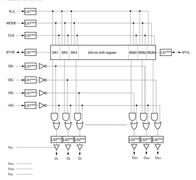
Note LS1: shifts CMOS level and internal level, LS2: shifts interval level and output level (VDD2-VEE).
